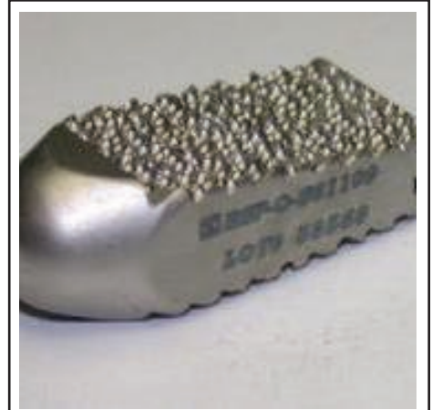
Two cervical spinal spacers are textured with the Tecotex I104 pattern.
